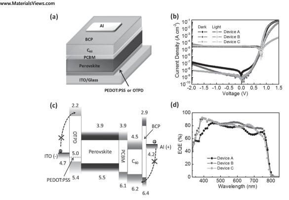
Figure 1. a) The schematic device structure of perovskite photodetectors. b) The dark current (solid symbols) and photocurrent density (hollow symbols, under white light  $\approx 143~\mu W~cm^{-2}$ ) versus bias curves of Devices A (diamonds), B (circles), and C (squares). c) The energy diagram of the perovskite photodetectors. d) The EQE curves of Devices A (circles), B (squares), and C (diamonds) at -0.1~V with the incident light modulation frequency of 35 Hz.
